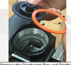
4.) Remove the Diaphragm Ring and DiaphragmAssembly.5.) Remove any dirt or debris from the body.Make sure all components are clean.
