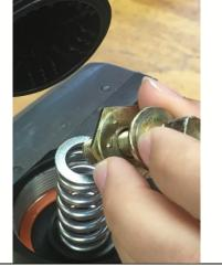
3.) Remove the Adjusting Bolt and Spring.
