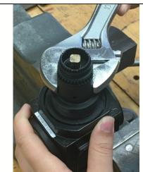
2.) Place the Piggyback Body in a vise. Use a wrench to gently remove the Bonnet.
