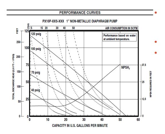
Use curves to determine if a pump can meet the application requirements
