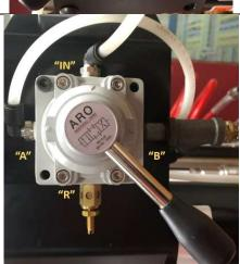
Rotating the lever to the right, actuates the "A" port.
