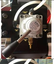
Rotating the lever to the left, actuates the "B" port.
