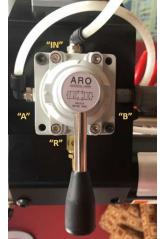
The M512LR is a 3-position, 4-way valve. All ports blocked in neutral.
