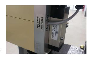
However, the **016414** is structurally different. The **M213SS-120-A** has 3/8" female threaded ports for the input, exhausts and both outputs. While the **016414** has threaded ports for the air inlet and two exhausts, the output ports are not threaded. They mate against the body of the dryer. O-Rings are used to seal the output ports.
