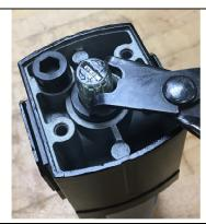
Use a spanner to remove the Sight Dome Housing.
