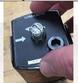
Reinstall the Upper Cover into the Lubricator Body.
