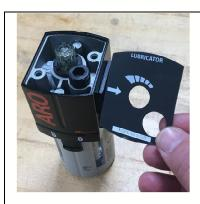
Relieve all air pressure in the system. Remove the Cover from the Lubricator Body.
