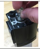
Install two Sight Domes into Lubricator Body
