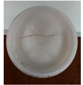
Example of chemical attack on a Delrin Plug
